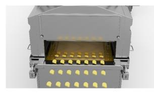
immersed. The built-in slot filter removes floating sediment from the fryer.
